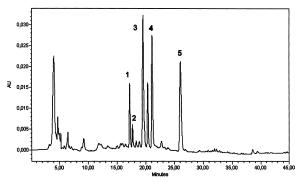
Fig. 2. UV chromatogram of a typical soy isoflavone extract obtained using 0.5 g of sample and 70% EtOH at 60 °C for 10 min. 1—Daidzin, 2—glycitin, 3—internal standard (2,5-dihydrox-ybenzaldehyde), 4—genistin, 5—malonyl genistin.
